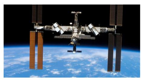
The International Space Station is powered entirely by 3000 square meters of solar panels that generate 246 kilowatts of electricity. Why solar? Because of its very low maintenance, extreme reliability, and the unlimited solar fuel delivered free of charge forever.
